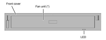
\*: You can see the fan unit by removing the front cover.
